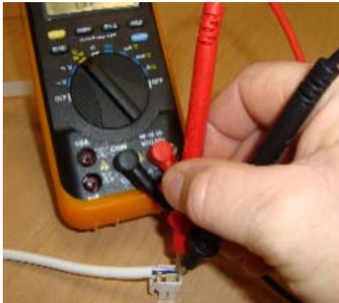
Checking the tact switch
